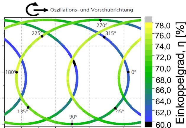
Figure 1: Change of the coupling ratio due to local power modulation
