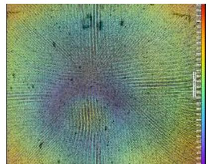
For joint welds on steel materials it could be shown that an estimation of the mechanical properties is possible by in-situ measurement of the phase transition temperature. By measuring during the welding process, a local prognosis of the property distribution can already be given, so that in the future a compensation is possible.
