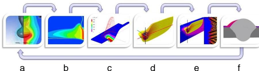
Fig. 1 Sub-areas of arc welding: (a) electrode wire and droplets, (b) arc, (c) drop zones (d) molten pool with free surface (e) solidification (f) weld seam.
