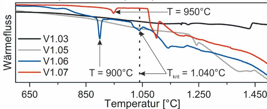
Figure 2: DSC results of master alloys
