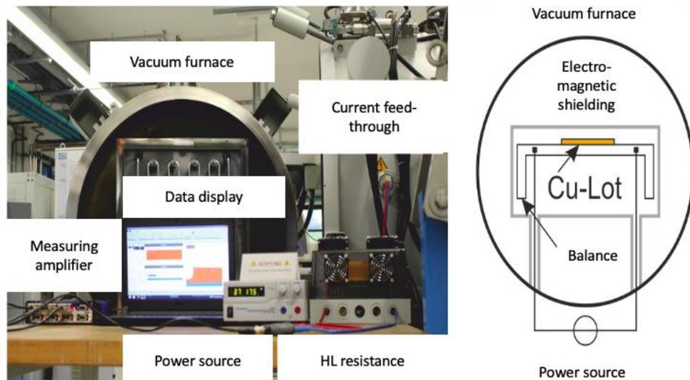
Figure 3: Experimental test rig for current-assisted soldering
