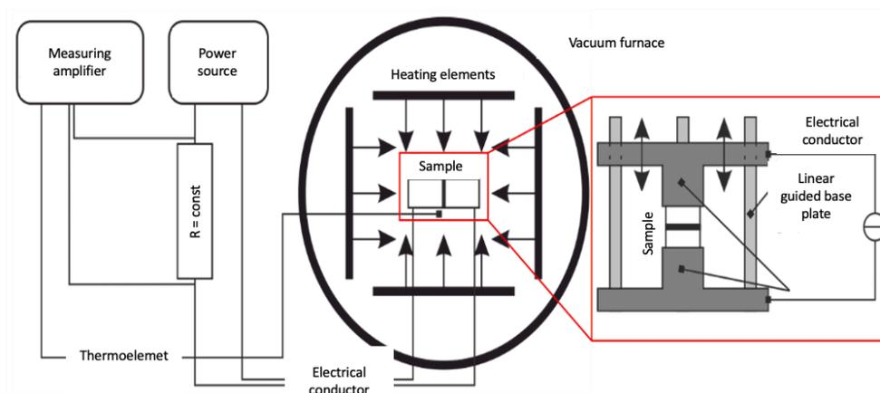
Figure 1: Schematic diagram of the experimental test stand at the Institute of Surface Technology
