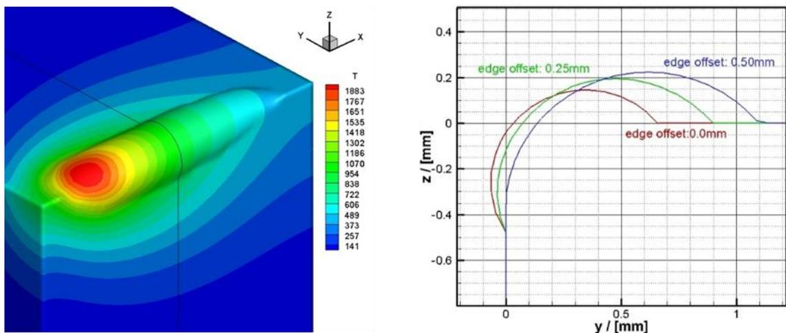
Figure 2 left: Calculated geometry and temperature distribution for LMD, right: calculated edge throw-up as a function of the edge offset (distance of the processing path to the edge)
