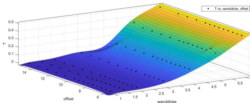
Figure 4: Relationship between optimization quality, wall thickness and tool offset
