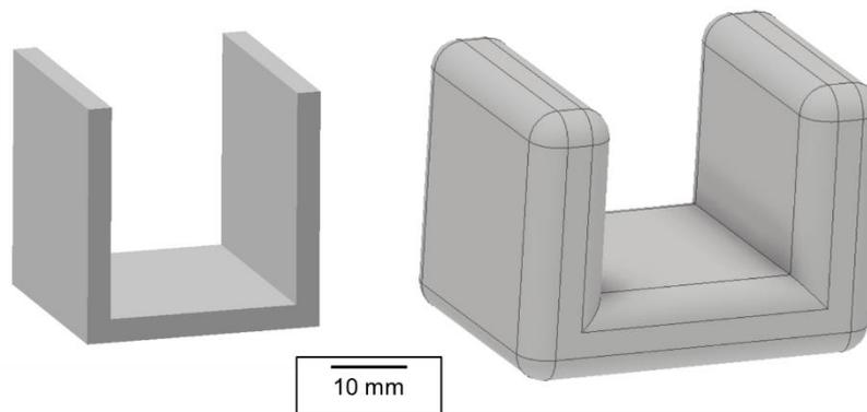
Figure 2: Simple example component and offset geometry of 6.5mm
