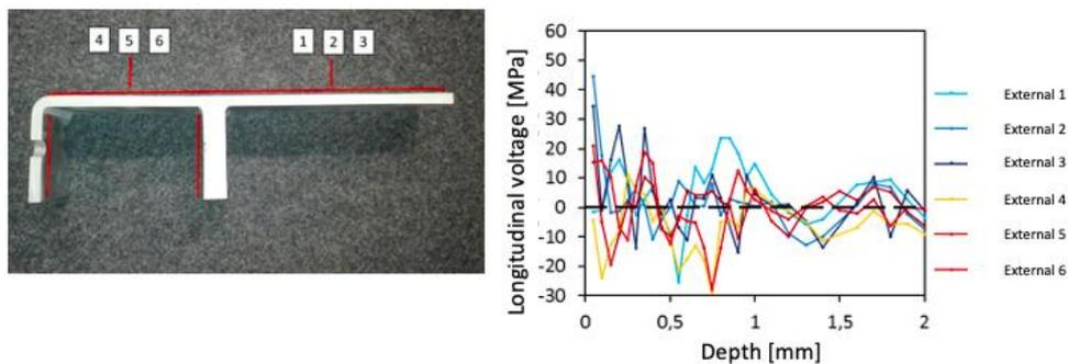
Fig. 7 Cut open complex test component with red marked measuring points for distortion measurement and numbered measuring points for the residual stress measurements (left). On the right side the corresponding residual stresses are plotted over the depth.
