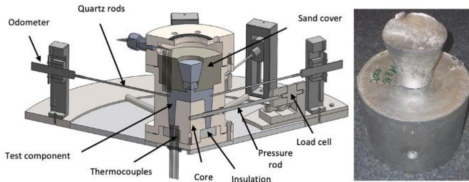
Fig. 2 Sectional view of the test stand for a rotationally symmetrical test component for HTC determination (left) and a corresponding cast test body (right)
