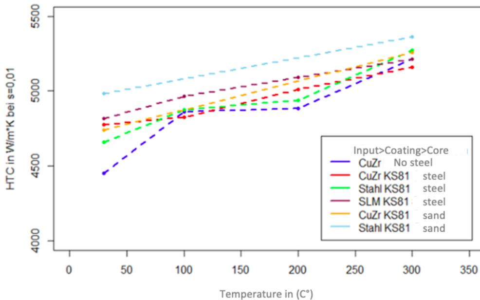
Fig. 6 Influence of the mould material and the cooling channel geometry on the HTC applied via the mould temperature control.
