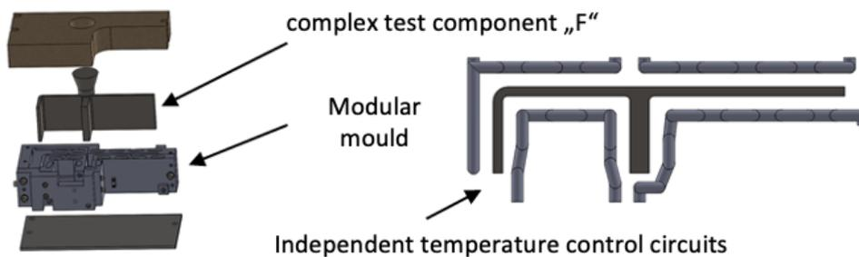
Fig. 3 Design of the test mould for the complex test component "F" (left) and arrangement of the individual temperature control circuits (right).
