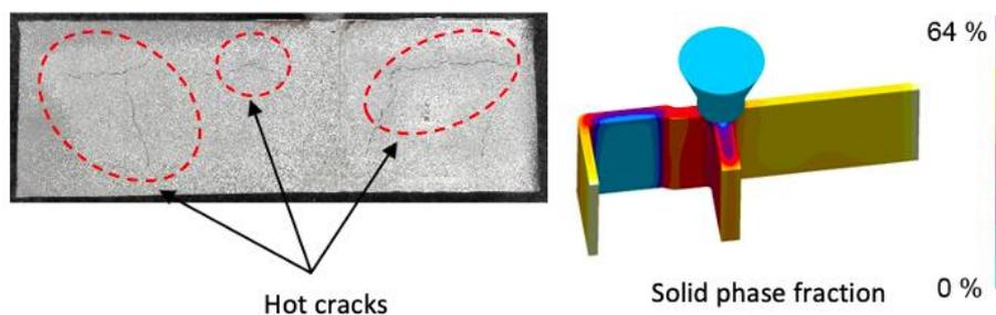
Fig. 4 Hot cracks generated in preliminary tests (left) and controlled solidification in an accompanying simulation (right)
