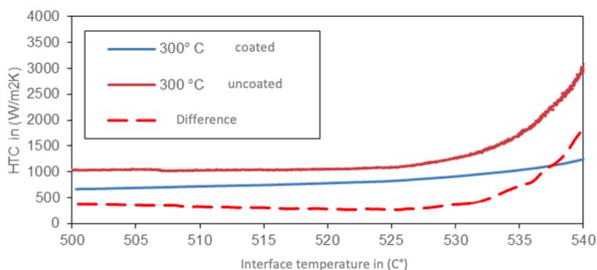
Fig. 5 HTC in a coated and an uncoated mould and the influence of the coating applied on the cast side Interface temperature
