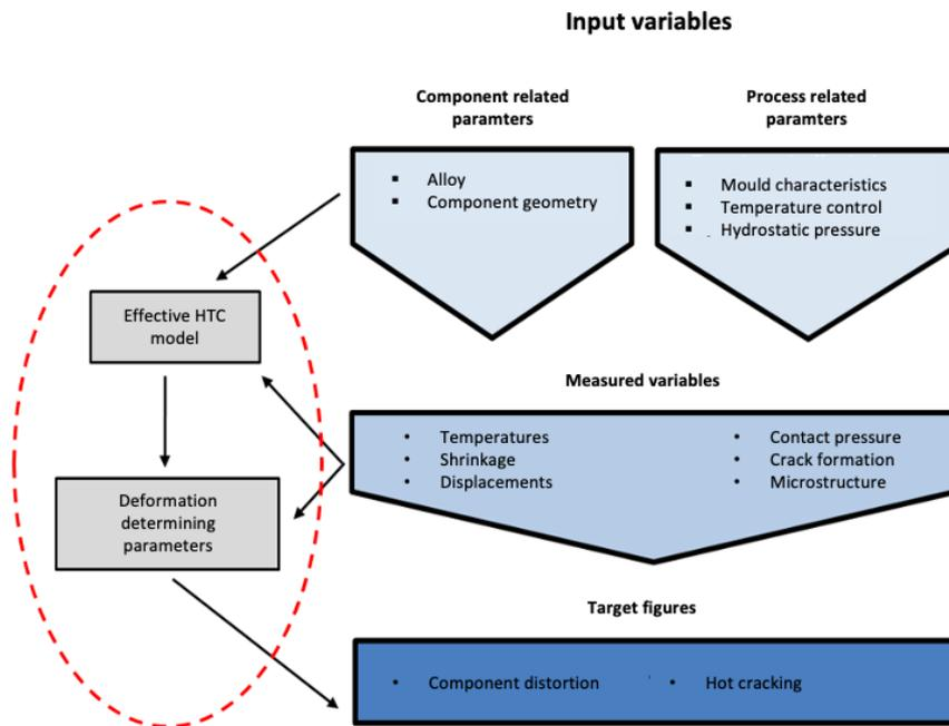
Fig. 1 Input, measurement and target variables and their interrelationships. The areas addressed in the subproject are marked.
