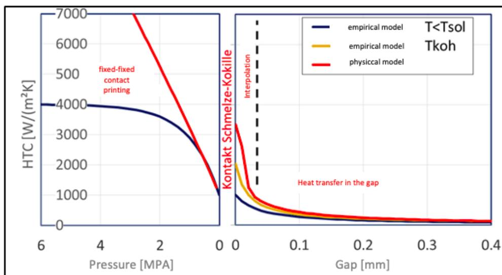
**Figure 2:** HTC curves of the empirical and physical heat transfer model for the case of contact pressure and gap formation
