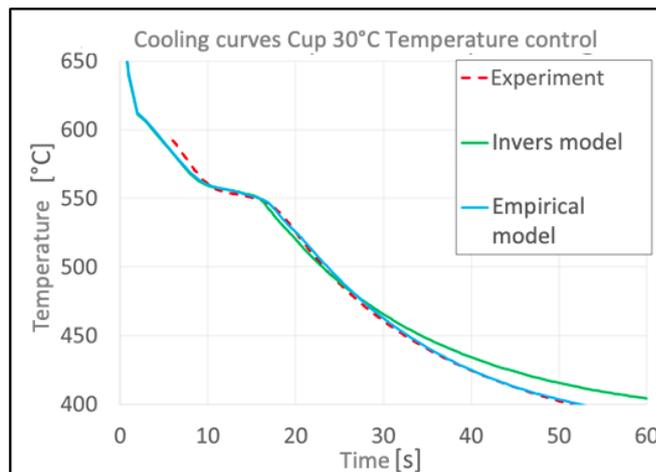
**Figure 4:** Cooling curves for inverse and empirical HTC model and measured values from experimental measurement
