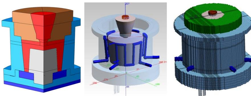
**Figure 1:** Left: Schematic diagram of the experimental setup (casting red, moulds light blue/grey, insulation dark blue, sand brown)
