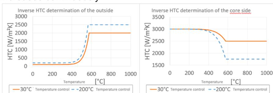
**Figure 3:** HTC(T) Progressions from the inverse simulations for two temperings of the setup
