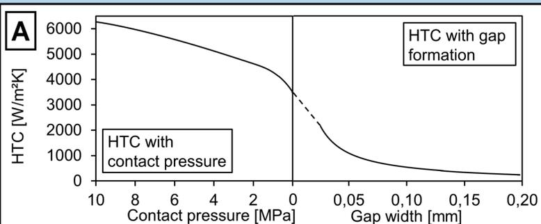
Pressure- and gap-dependent heat transfer coefficient as solid-solid contact
