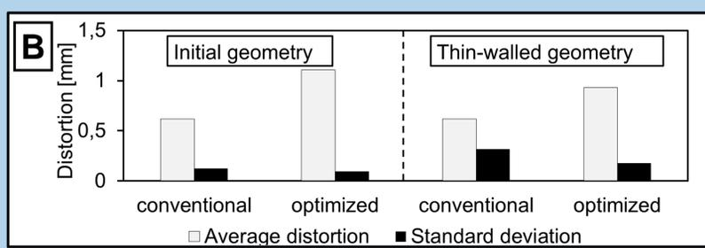
Mean component distortion and standard deviation for conventional mold modules and those with optimized cooling for different component geometries
