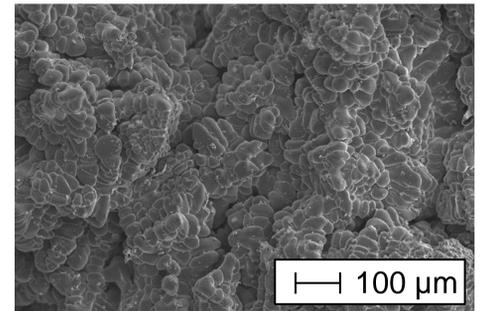
In-situ detection of a hot tear in AlSi1.75Mg and images of its morphology at different scales
